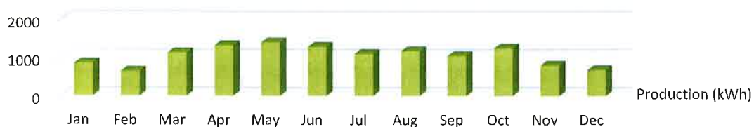
Aurora Solar Production Simulation 12,731 kWh
