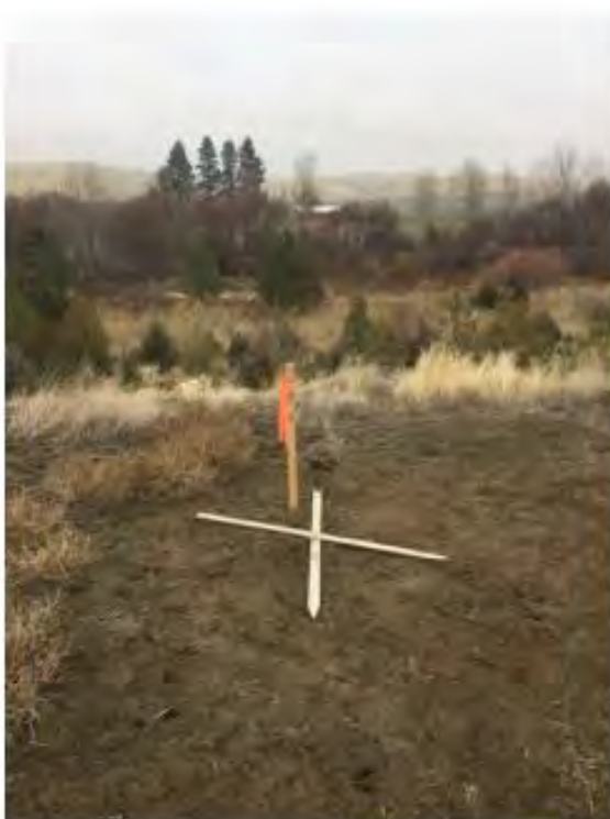
31- Stake location is CP56 approximately 250ft upstream perpendicular from existing bridge. To capture river valley survey.
