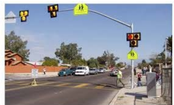
Figure 28. Example of a HAWK system
