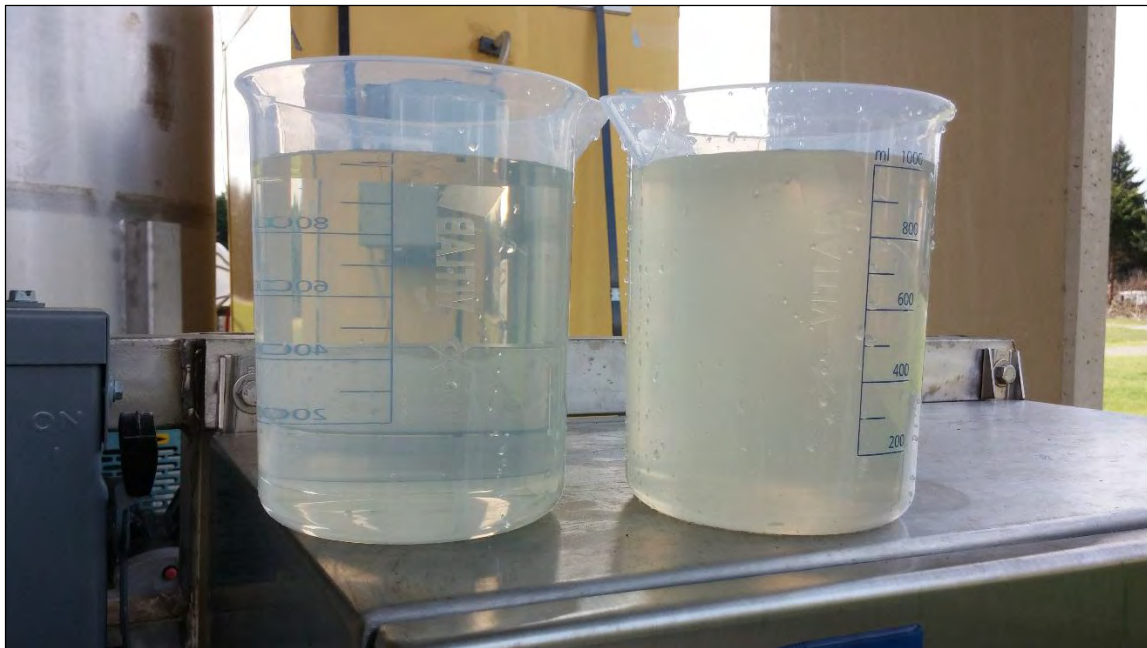
Photo of Pilot Filter Effluent (Left) and Pilot Filter Influent (Right)
