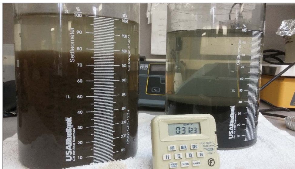
Photograph ES-9. Gravity SBR Sludge Settling (Left) versus Ballasted Sedimentation Assisted Settling (Right)
