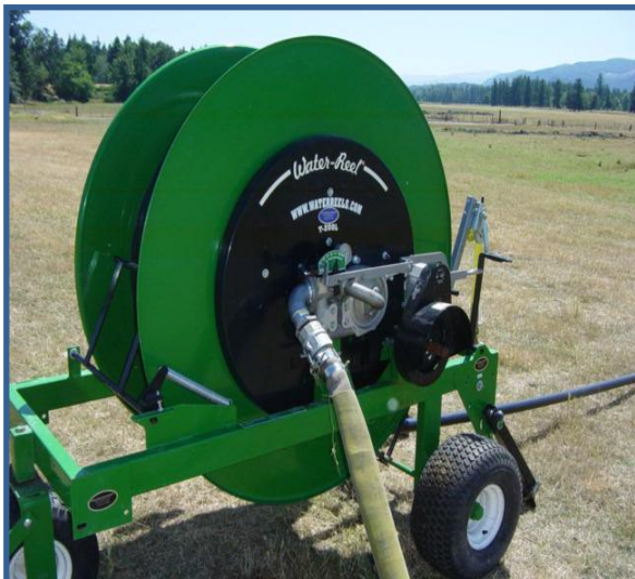
Photo C Smith irrigation Water Reel with 2 inch diameter hose
