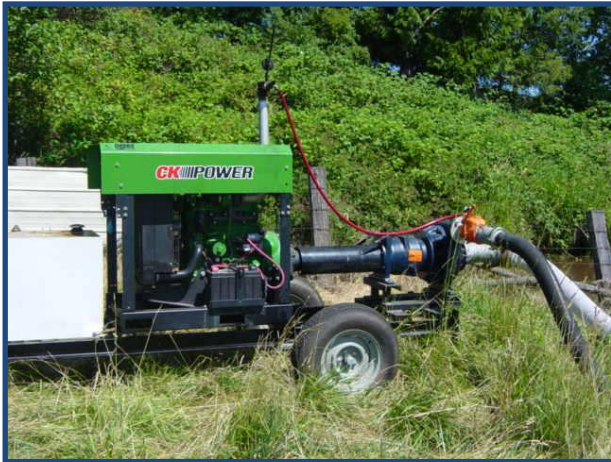
Photo A John Deere diesel motor and NACD Pump with suction hose and delivery to Reel
