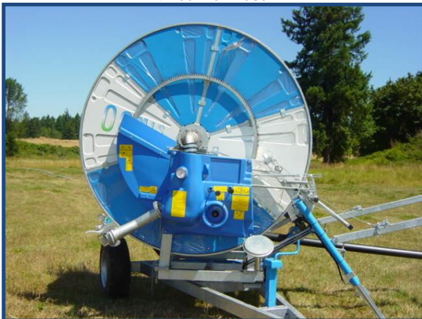
Photo C OCMIS Water Reel with 1,148 feet of three-inch hose
