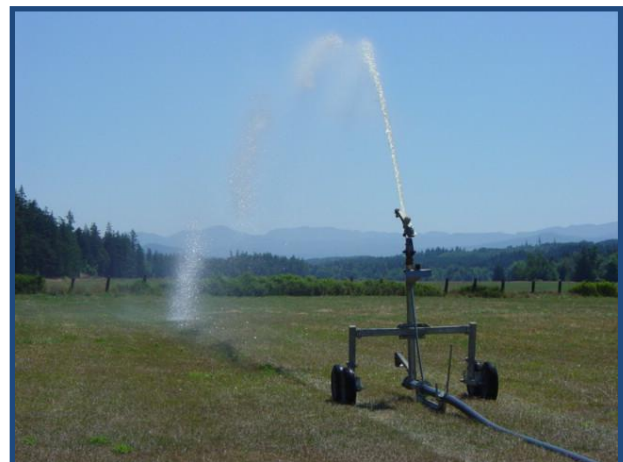
Photo D Big Gun with two-inch nozzle irrigating NE portion of the 135 acre POU
