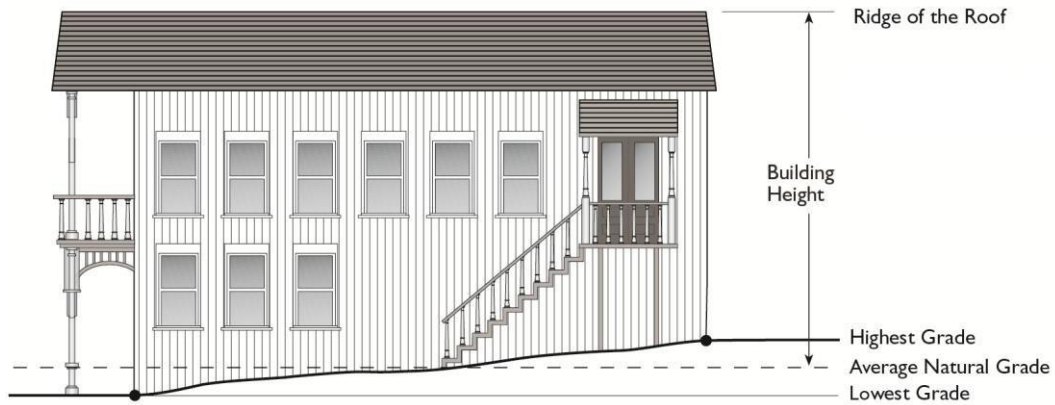
FIGURE 11.03.050(A): MEASURING BUILDING HEIGHT
