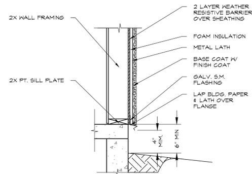
TYP. ONE COAT STUCCO EXTERIOR DETAIL
