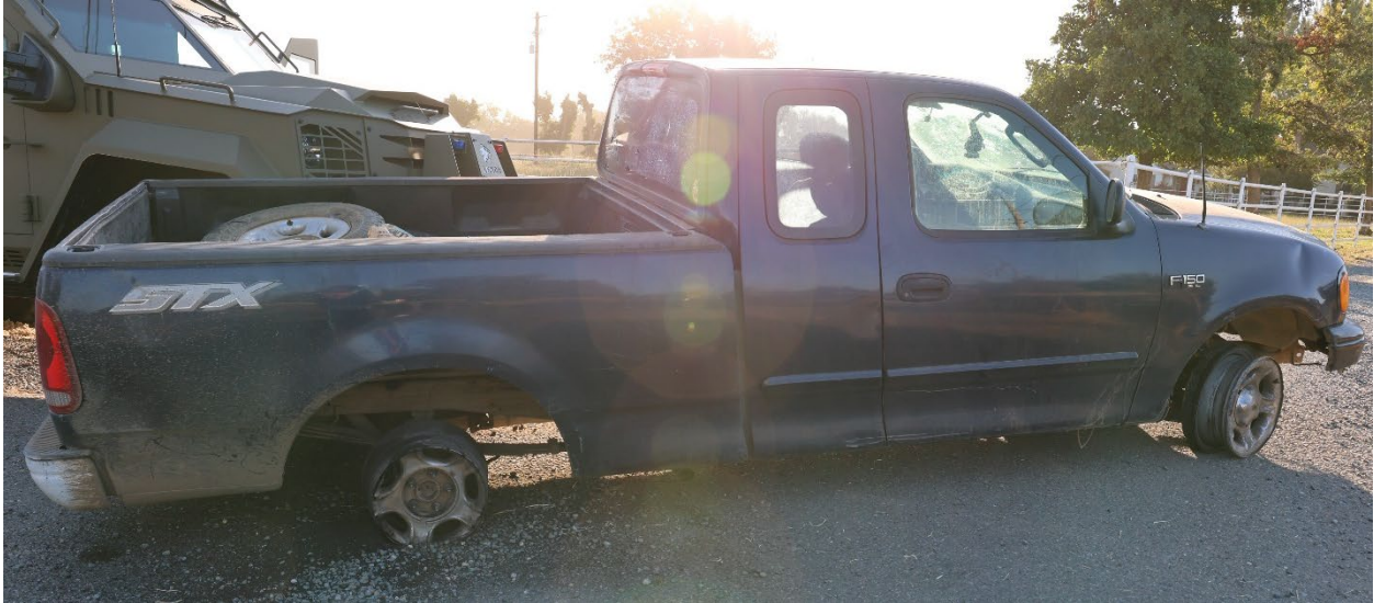
Figure 008 – Photo taken by DOJ personnel, showing the passenger side of the truck. Notice the tires were completely gone, and the barrel of the rear wheel is nearly flat.
