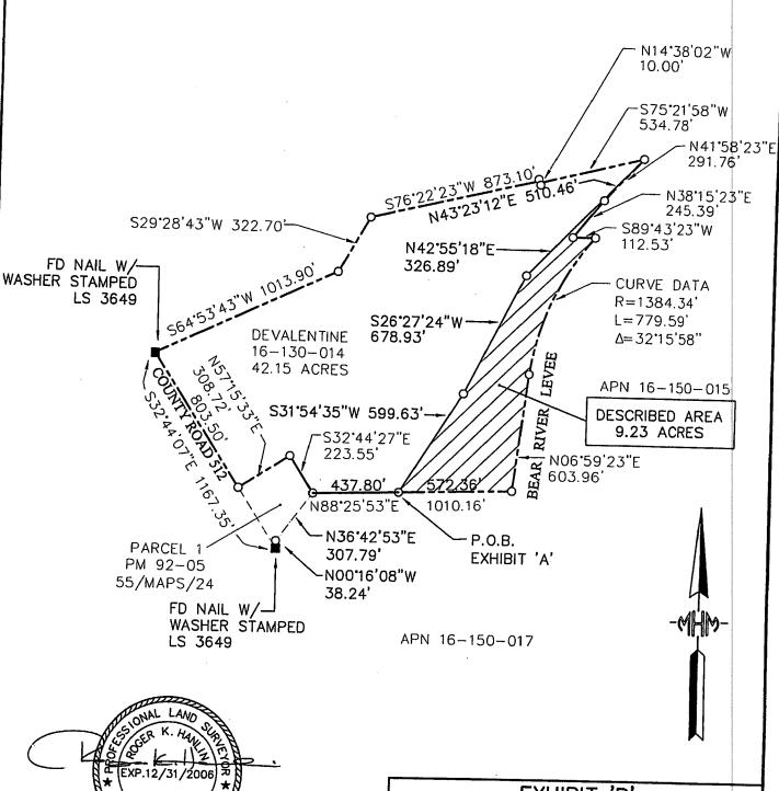
BEARINGS SHOWN HEREON ARE BASED UPON THE CALIFORNIA COORDINATE SYSTEM, ZONE 2, NAD83, 1986 EPOCH AND ORIGINATE FROM THE CONTROL SURVEY FILE NO. 03—25F BY THE U.S. ARMY CORPS. OF ENGINEERS IN OCTOBER 2003.
