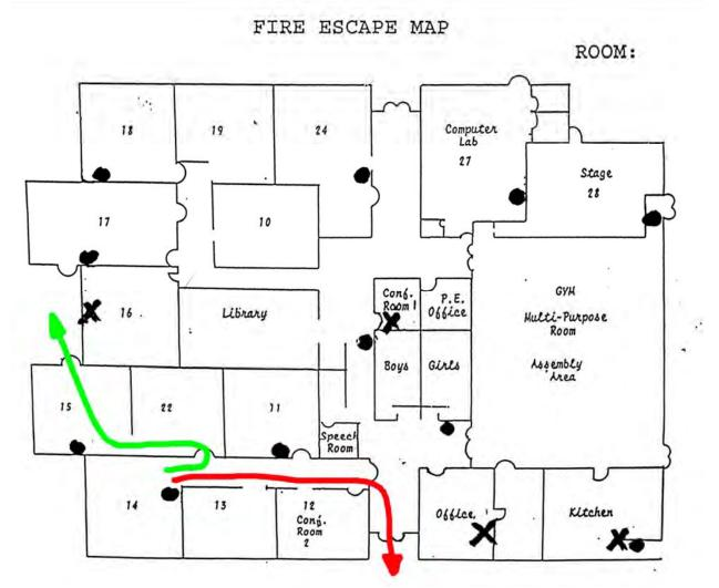
**Figure 2.** Fire Escape Map for some of the classrooms at Foothill Intermediate School. The emergency escape route from room 14 practiced during school drills is shown in red. The alternate route, suggested by the Grand Jury, is shown in green.
