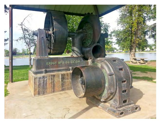
**Figure 4.** In 1895 Pumps were installed at the confluence of the Yuba, and Feather Rivers, to protect the city of Marysville from the danger of flooding and were powered by high capacity electric motors.
