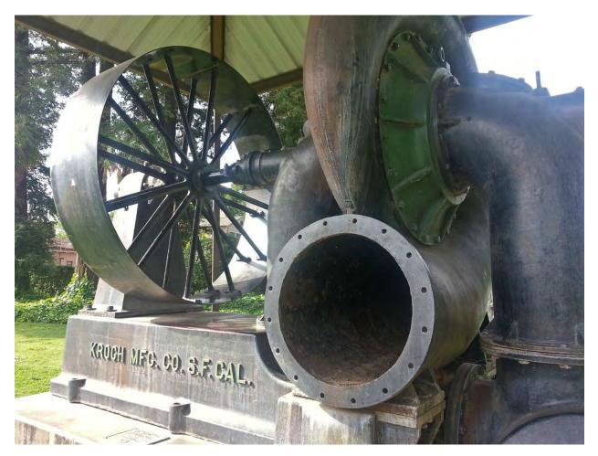
**Figure 5.** *These pumps have a capacity to pump 18,265 gallons per minute. That's approximately equal to the capacity of the average back yard swimming pool, each minute.*
